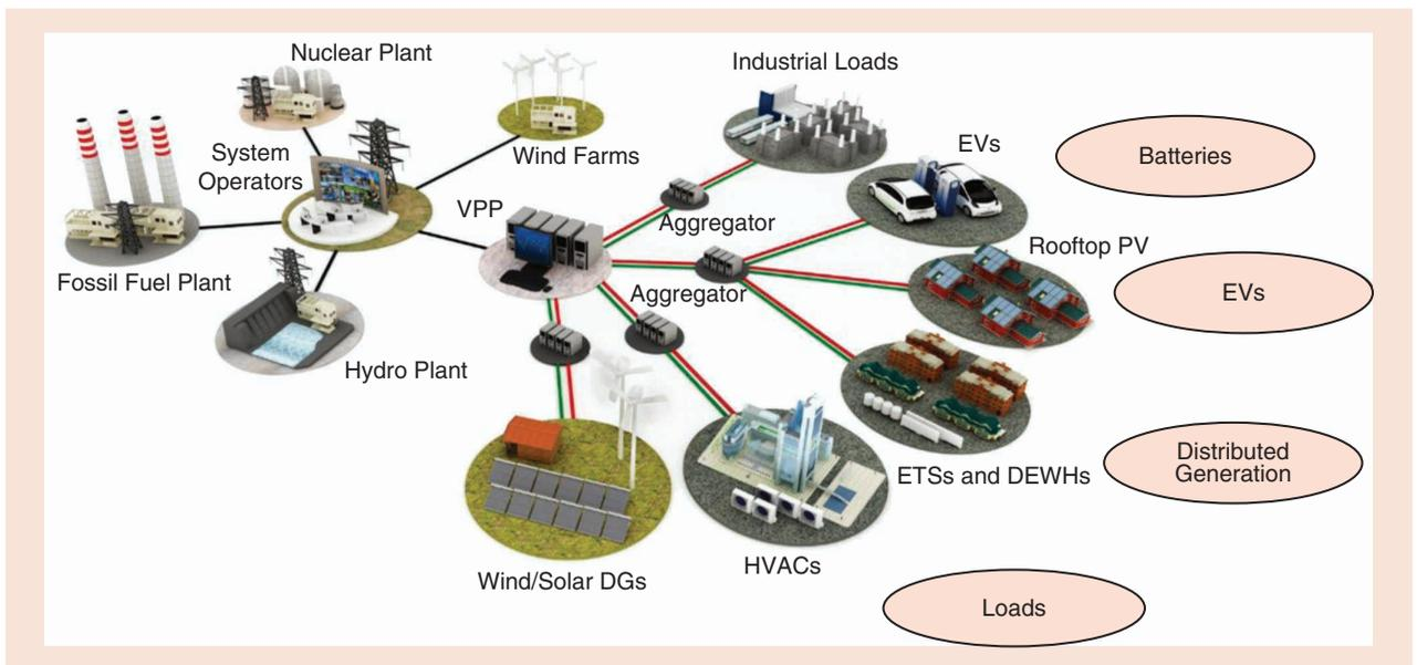
**FIG 2** The demand-side management of thermal loads as part of the DERs portfolio. DG: distributed generator; HVAC: heating, ventilation, and air-conditioning; VPP: virtual power plant; ETS: electrical thermal storage; DEWH: domestic electrical water heater. (Source: Prof. Liuchen Chang; used with permission.)
